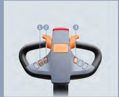
FREI Multi-Function Tiller 1: Forks move forward / backward 2: Lifting / lowering of forks 3: Forward / backwards tilting of forks
