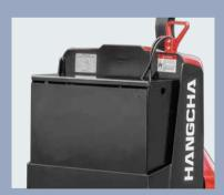
The battery compartment is sized to fit either a 12-85-5 industrial battery in its 7.8 inch compartment for heavier throughput applications
