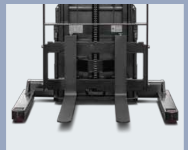
Fixed Straddle Baselegs ( Inside Dimension in 4" increments from 38" to 50"); Adjustable baseleg optional to fit a wide range of pallet sizes
