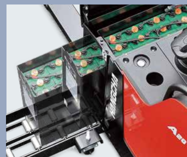
Side battery change is standard feature
