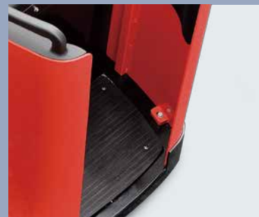
The pedal applies shock absorption design, greatly improve the operator's comfort, reduce the fatigue
