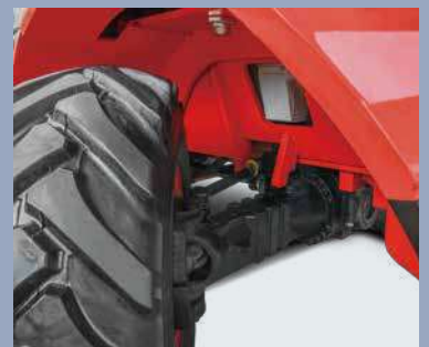
Oscillating steer axle allows either wheel to step over obstacles keeping the truck and load level
