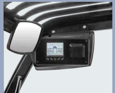
Large screen display, the instrument panel adopts injection molding design, sturdy and durable
