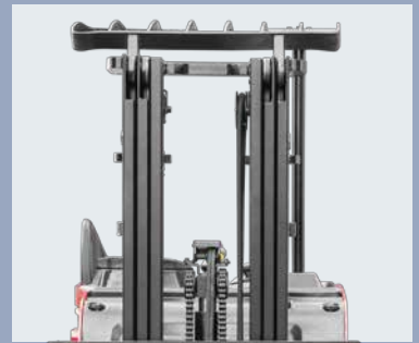
Wide mast provides perfect visibility and hydraulic cushioning provides confident and smooth load handling
