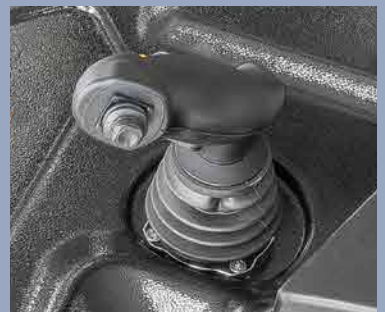
The intuitive, multifunction control handle is centrally positioned for easy access to truck functions and offers simultaneous control of drive, lift, lower and auxiliary hydraulic functions
